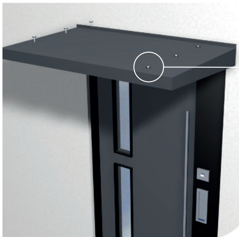
6. Slide assembled canopy onto the wall brackets until the canopy sits tight to the wall. Secure the canopy to the wall brackets using 6x self-tapping screws with rubber-washer (as shown).
